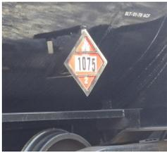
The Hazardous Material Placard showed 1075, flammable. It was determined through the app, that this car was carrying Propane. Public Safety factors and a Hazard Analysis was completed using the app.
